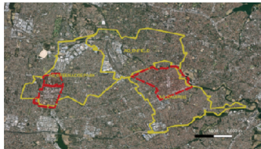
Figure 5 Relative coverage of zone substations supplying study areas
